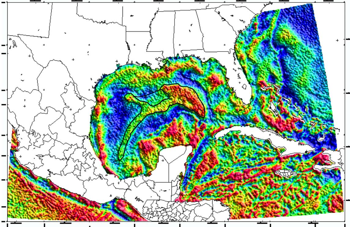
*Satellite-derived isostatic gravity anomaly in the Gulf of Mexico. The central positive anomaly correlates with true oceanic crust. Shoreward lies transitional crust, an area of highly attenuated often intruded, and relatively thin crust.*
